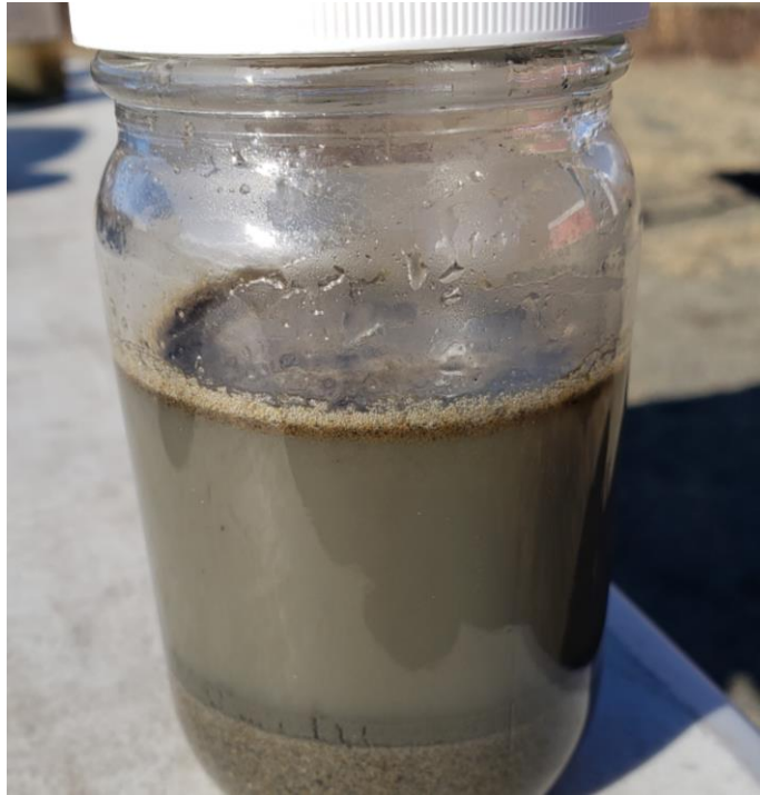
View of Failed Soil/Water Agitation Test within FPA-35 at 6.0 – 6.5.
