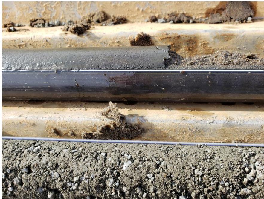
View of separate phase (product) on FPA-5 boring liner.
