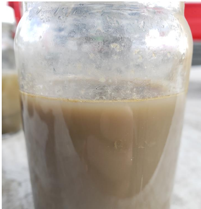
View of Failed Soil/Water Agitation Test within FPA-33 at 6.0 – 6.5 Feet.
