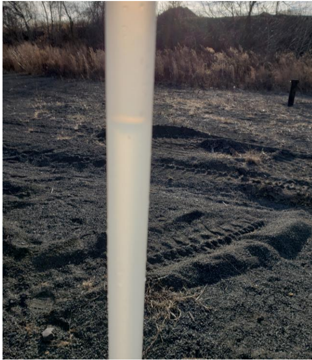
View of no measurable product on groundwater within TWP-30.
