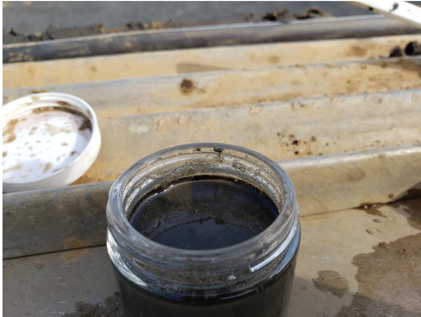
Close up view of Agitation Test Fail at FPA-7 (6.5 Feet).
