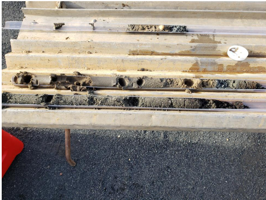
View of typical soil core (FPA-1 shown) from within the excavation area. The closer core represents 0 to 5 feet (excavation backfill) and the further core represents 5 to 10 feet with product saturated soils present from approximately 7.5 – 9.5 feet.
