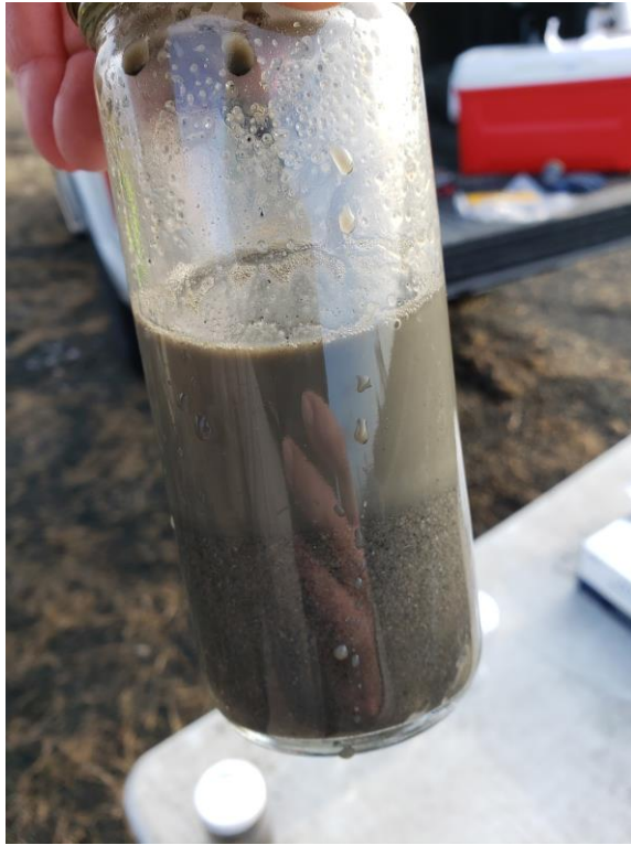
View of Failed Soil/Water Agitation Test in Boring FPA-25 at 6.0 – 6.5 Feet.
