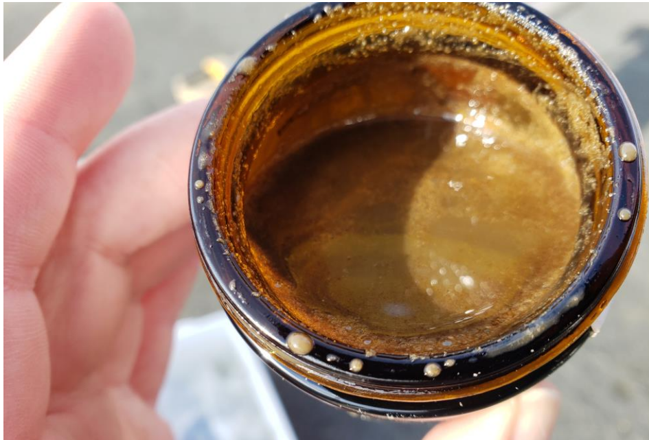
View of Failed Soil/Water Agitation Test at FPA-2 at 8.0 feet below ground surface.
