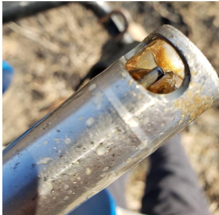
View of Oil/Water interface probe with oil globules on tip from TWP-5 (Boring FPA-5).
