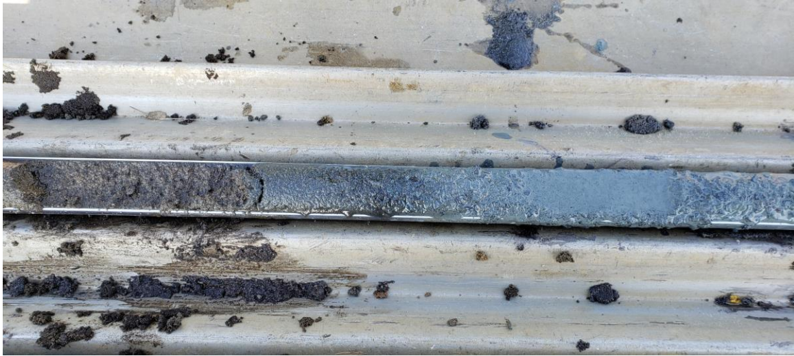
View of heavy petroleum impacts in soil boring FPA-28 from 7.0 – 9.0 feet.
