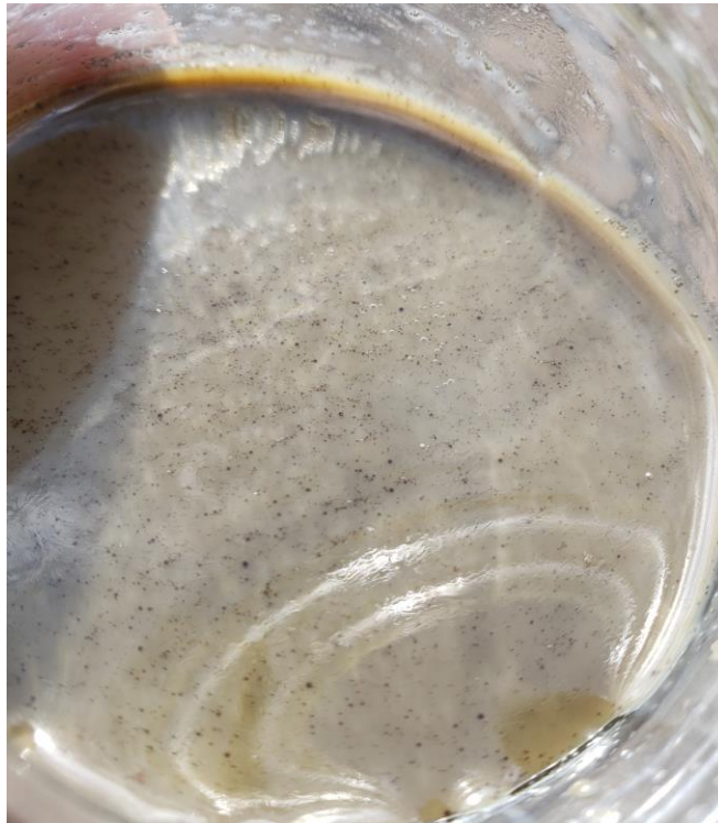
Close View of Failed Soil/Water Agitation Test in Boring FPA-32 at 6.0 – 6.5 Feet.
