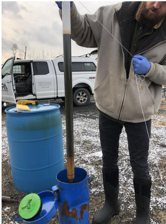
View of over two-feet of product in PR-1. An accurate measurement was difficult due to the amount of product present. (Photo taken on January 20, 2021)
