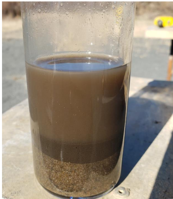
View of Passed Soil/Water Agitation Test at FPA-21 (8 Feet). Potential delineation point.
