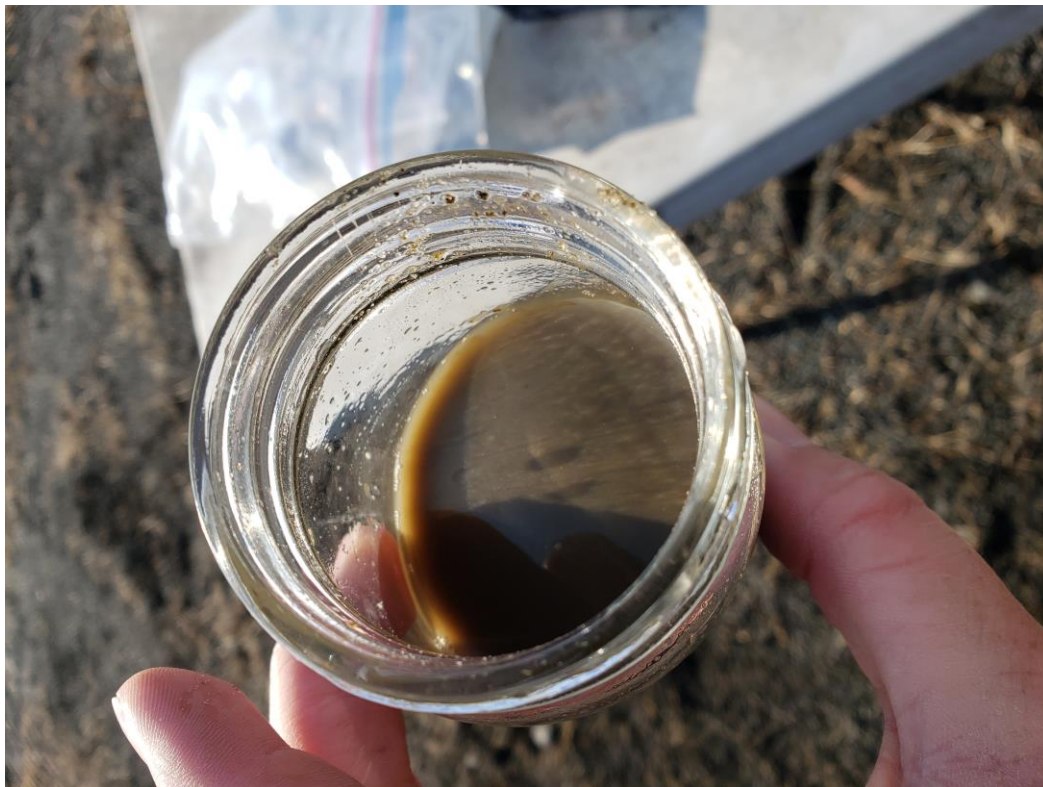
View of Passed Soil/Water Agitation Test in Boring FPA-27 at 8.0 – 8.5 Feet.
