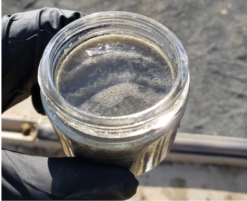
View of Failed Soil/Water Agitation Test at FPA-14 (Top View).
