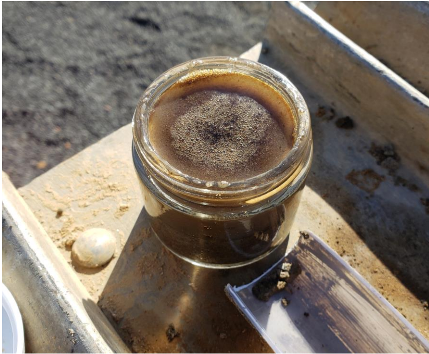
View of Failed Soil/Water Agitation Test at FPA-12 (8 Feet).
