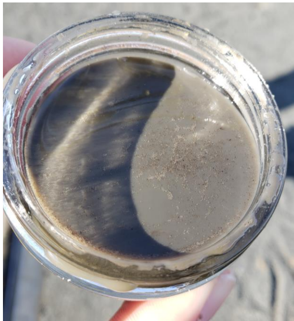
View of Failed Soil/Water Agitation Test at FPA-13 (8 Feet).
