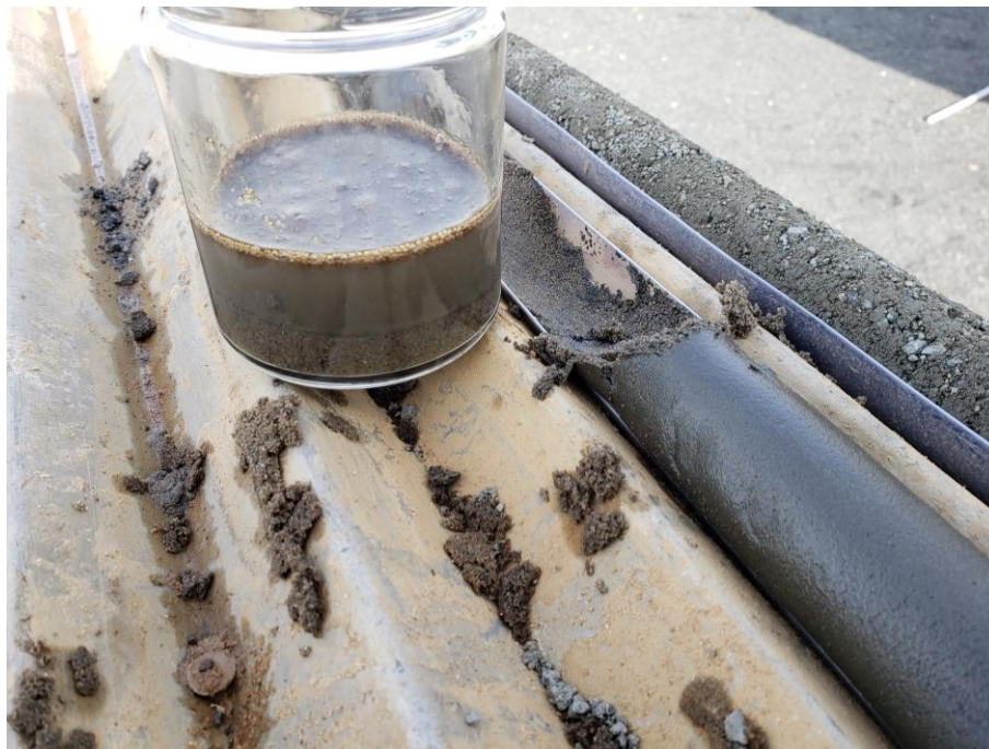
View of Failed Soil/Water Agitation Test at FPA-5, next to product saturated soils.
