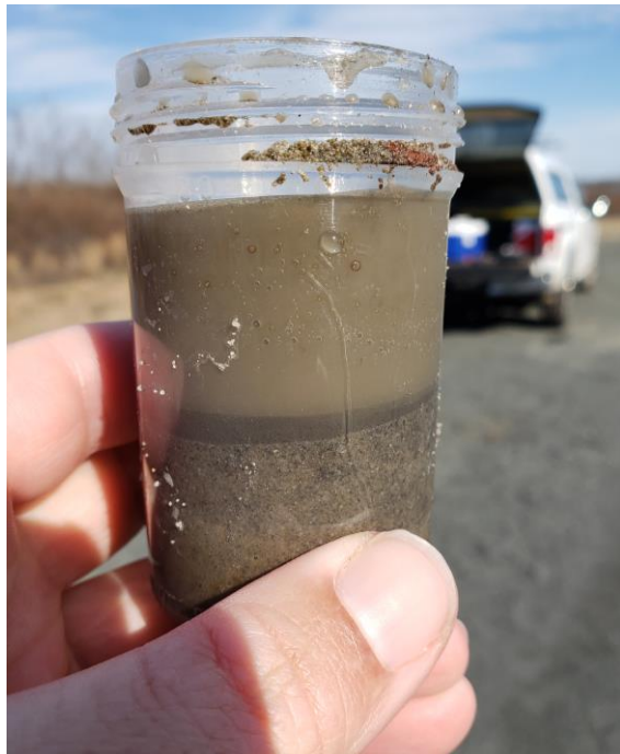
View of Failed Soil/Water Agitation Test at FPA-10. See oil globules trapped on the sides of the container.
