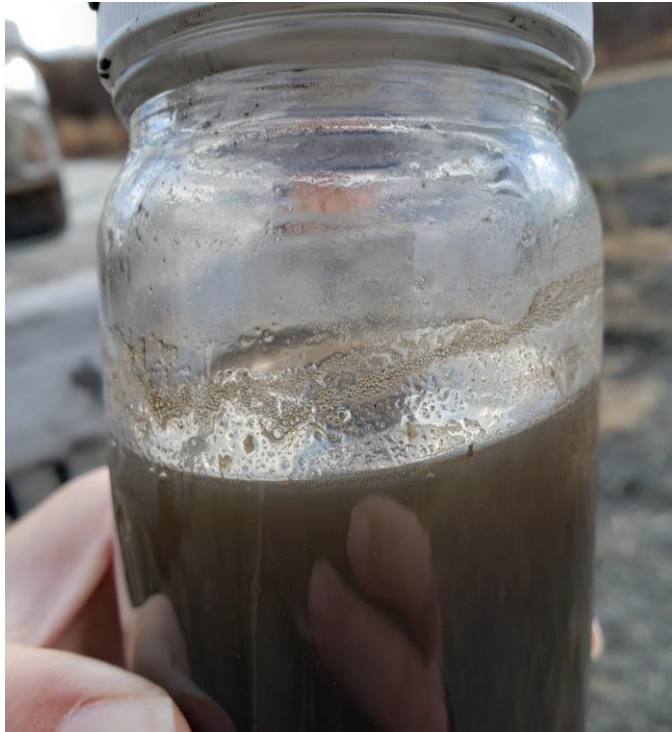
View of Failed Soil/Water Agitation Test within FPA-32 at 7.5 – 8.0.
