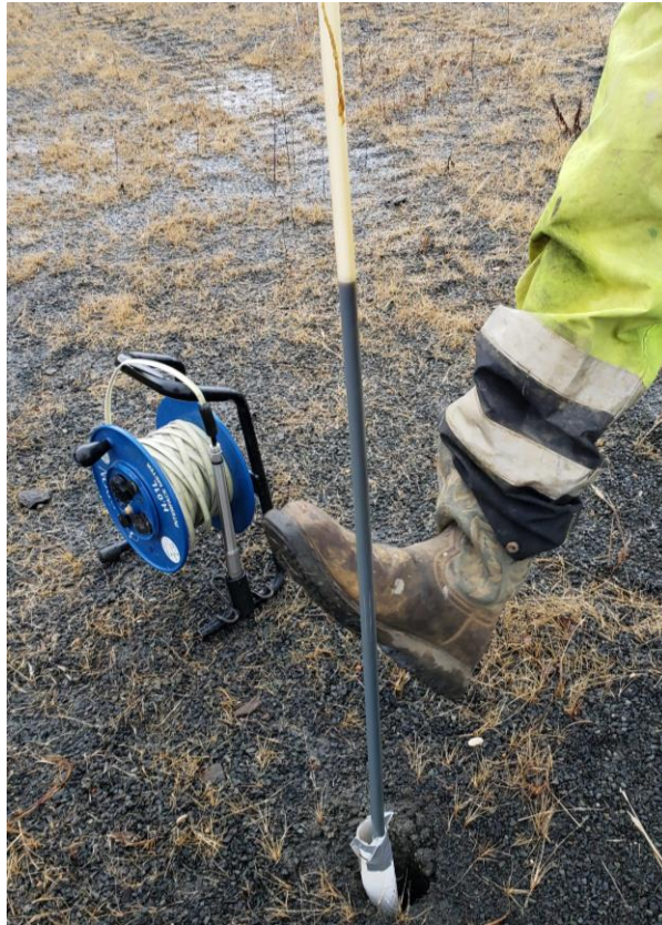
View of several feet of product in TWP-18 (Boring FPA-18). Just over two feet measured.
