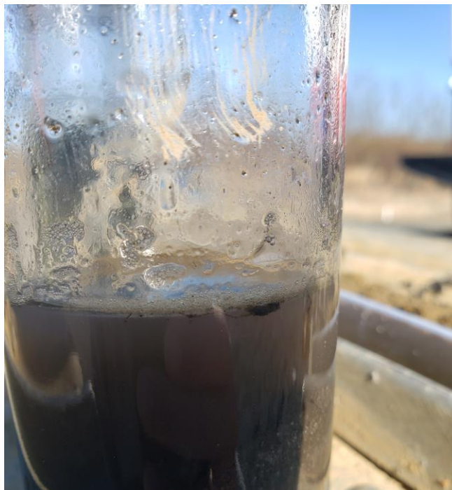
View of Failed Soil/Water Agitation Test at FPA-18 (8 Feet).
