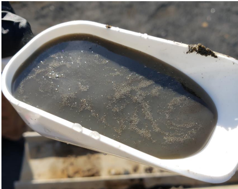
View of Failed Soil/Water Agitation Test at FPA-15 (6.5 Feet).
