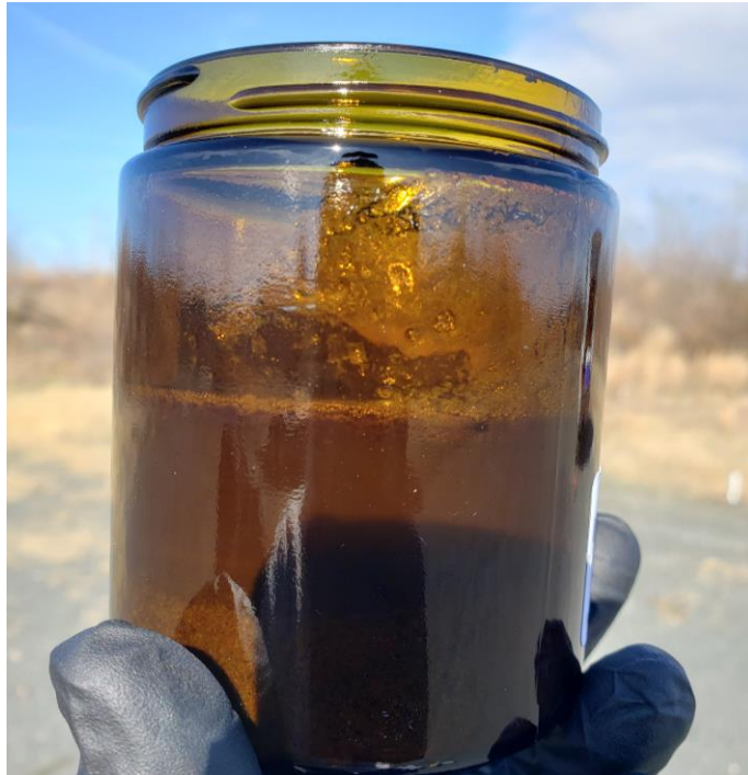
View of Failed Soil/Water Agitation Test at FPA-11 (7.5 Feet).
