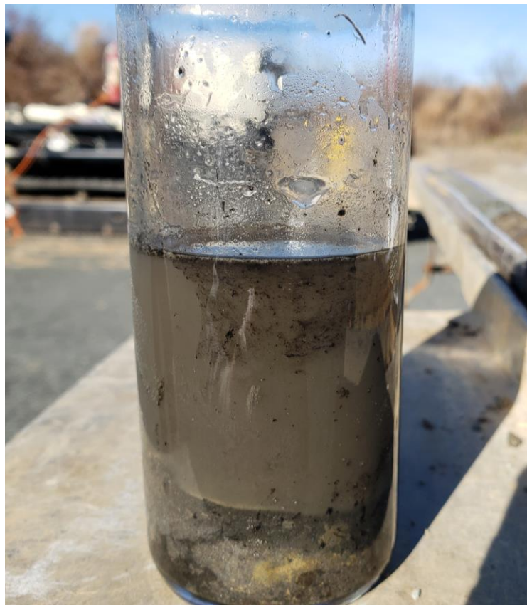
View of Failed Soil/Water Agitation Test at FPA-22 (7.5 Feet). Very Black product.
