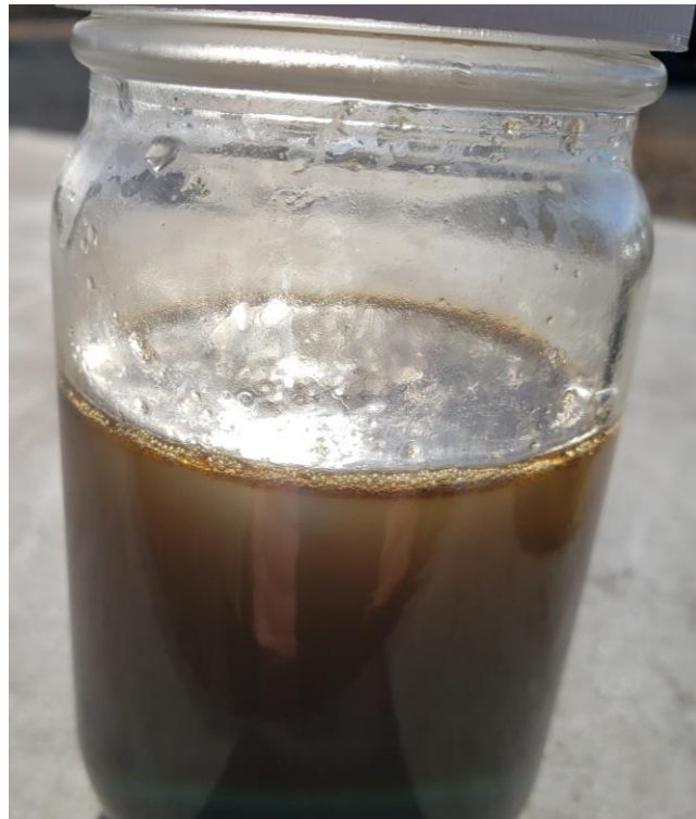
View of Failed Soil/Water Agitation Test within FPA-35 at 8.0 – 8.5.
