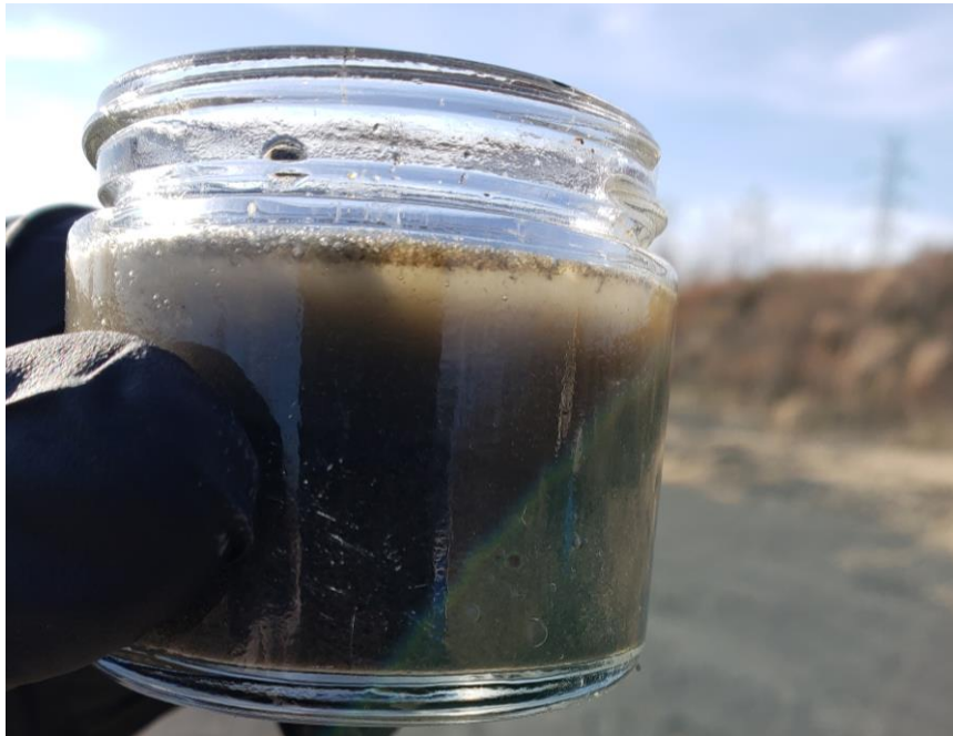
View of Failed Soil/Water Agitation Test at FPA-14 (8 Feet).
