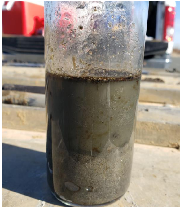
View of Failed Soil/Water Agitation Test at FPA-19 (8 Feet).
