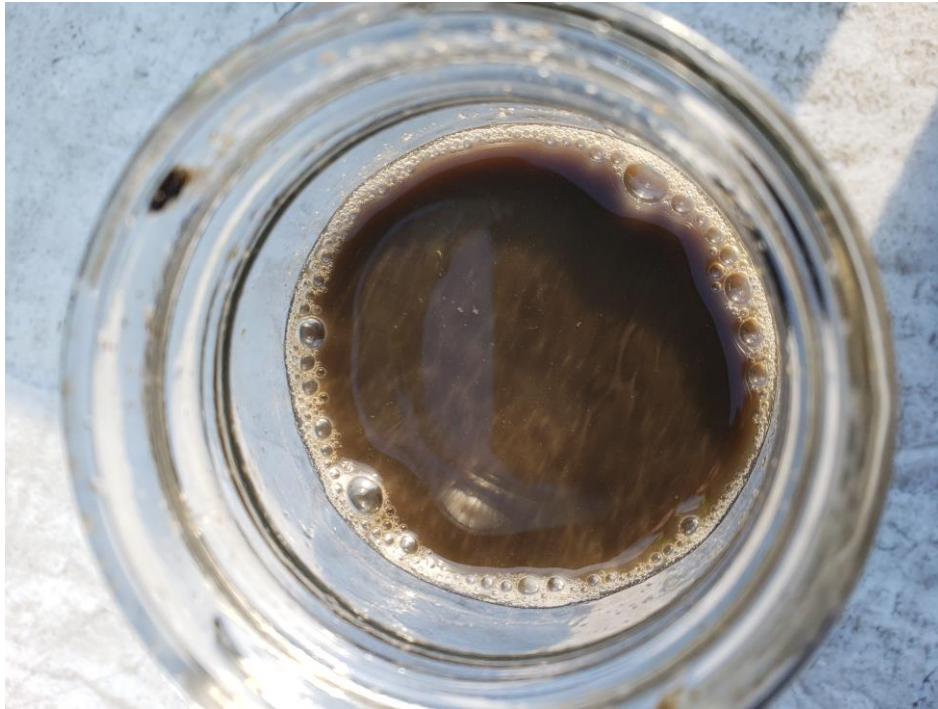
View of Passed Soil/Water Agitation Test in Boring FPA-26 at 7.5 – 8.0 Feet.
