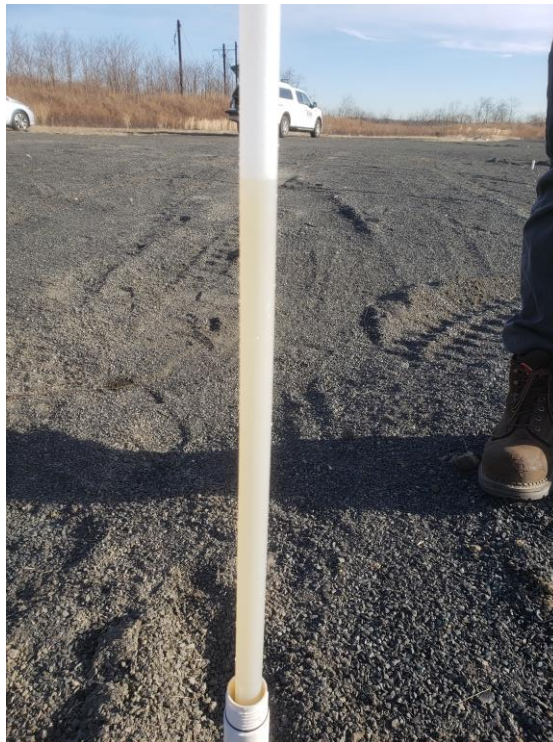
View of no measurable product on groundwater within TWP-32.
