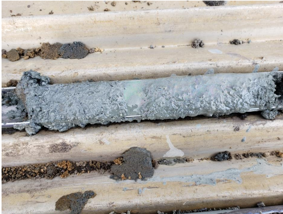
View of heavy petroleum impacts and sheen on water/soil within FPA-30 at 7.0 – 9.0 feet.
