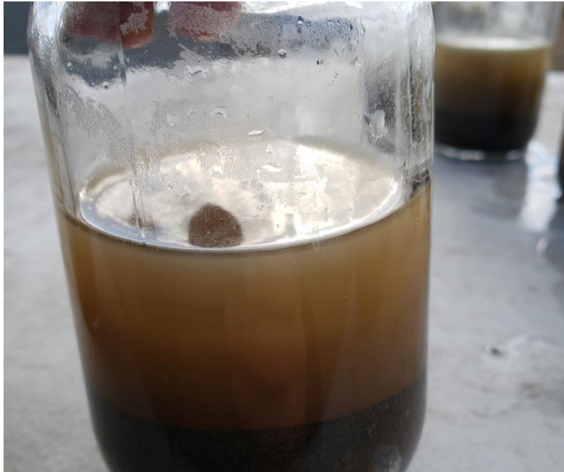
View of Passed Soil/Water Agitation Test within FPA-36 at 8.5 – 9.0.
