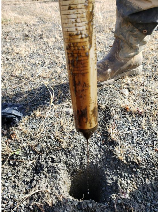
View of oil streaming off TWP-17 after removal.
