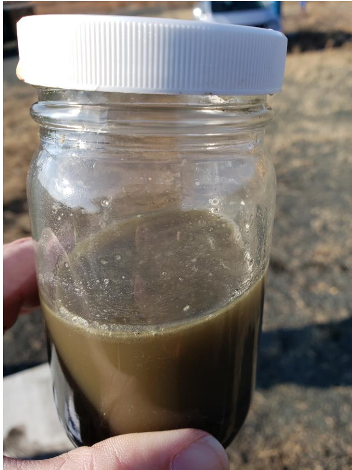
View of Failed Soil/Water Agitation Test in Boring FPA-28 at 8.0 – 8.5 Feet.
