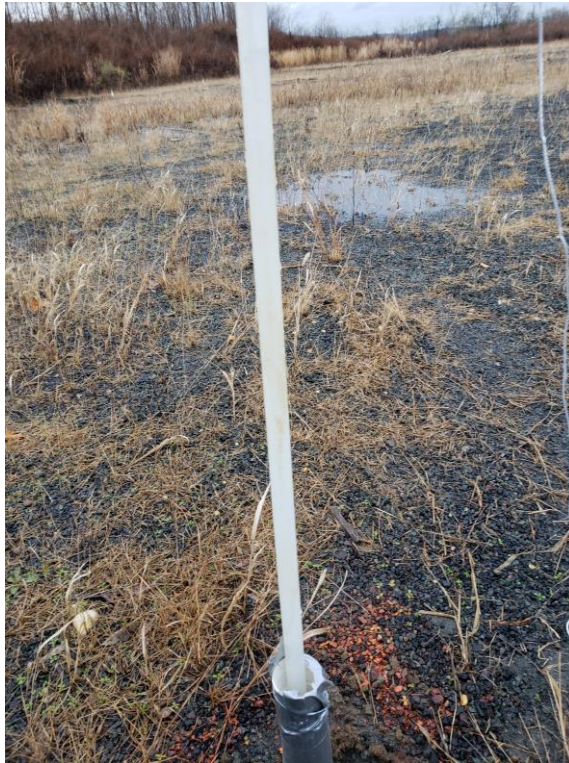
View of clean bailer (no measurable product) from TWP-1 (Boring FPA-1). Strong Petroleum odor noted on the groundwater.
