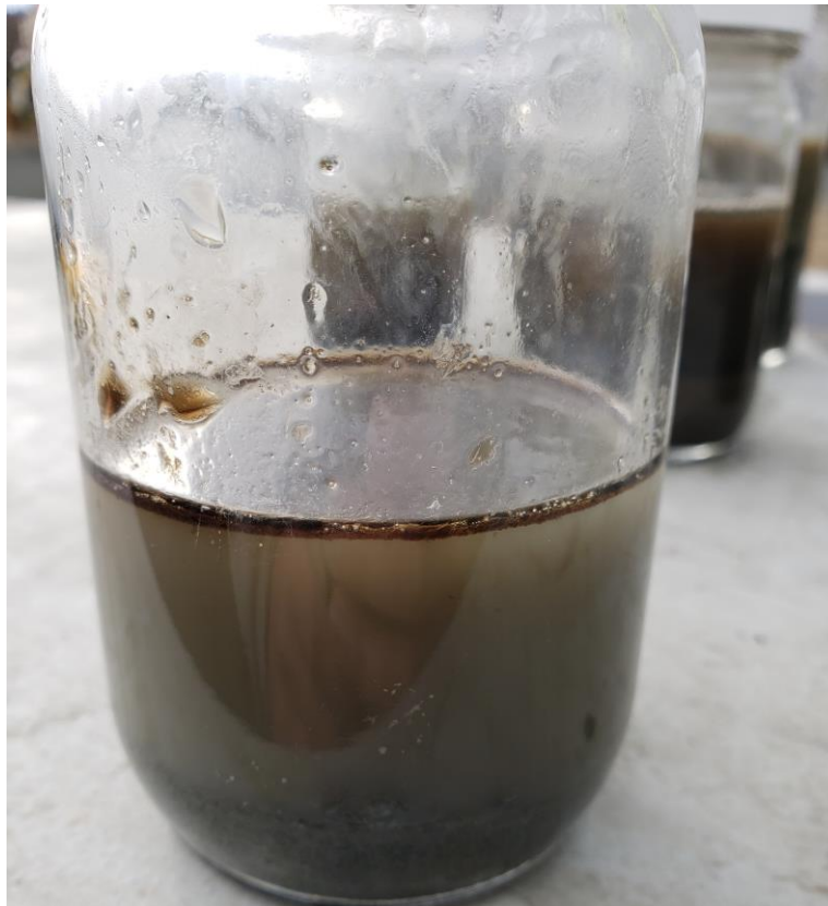
View of Failed Soil/Water Agitation Test in Boring FPA-30 at 7.5 – 8.0 Feet.
