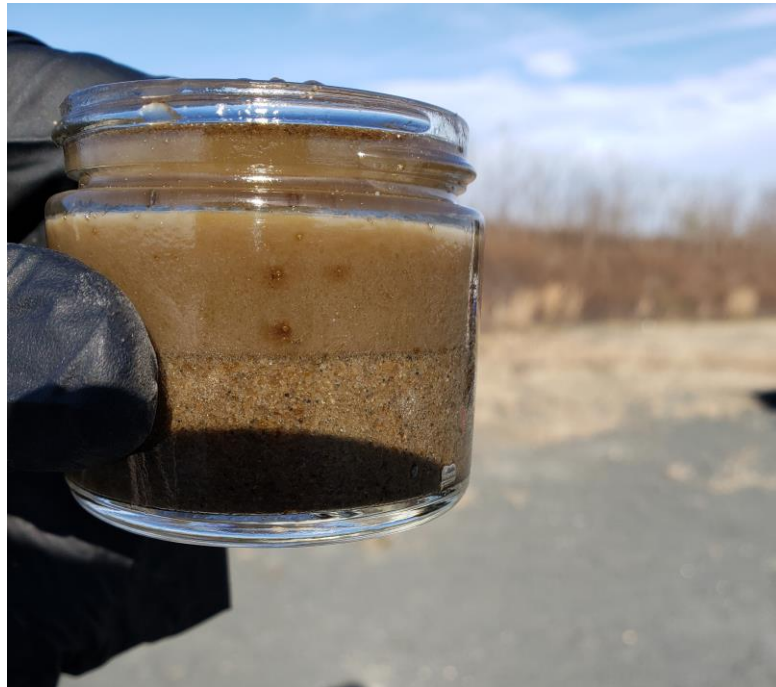
View of Failed Agitation Test at FPA-12. Side view to show separate phase still bound to the fine sands even when water is applied.
