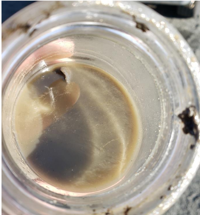
View of Passed Soil/Water Agitation Test within FPA-38 at 4.0 – 4.5 feet where heavy petroleum impacts were observed.
