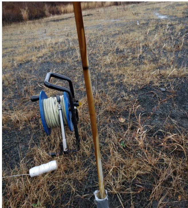
View of approximately one-inch of product in TWP-11 (Boring FPA-11).
