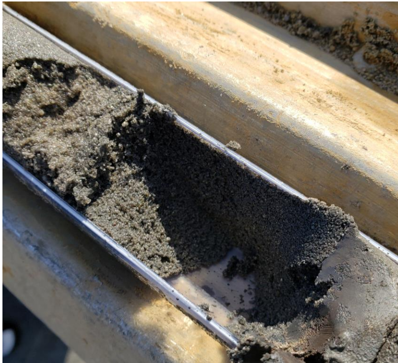
View of product saturated soils at FPA-14 (8 Feet).
