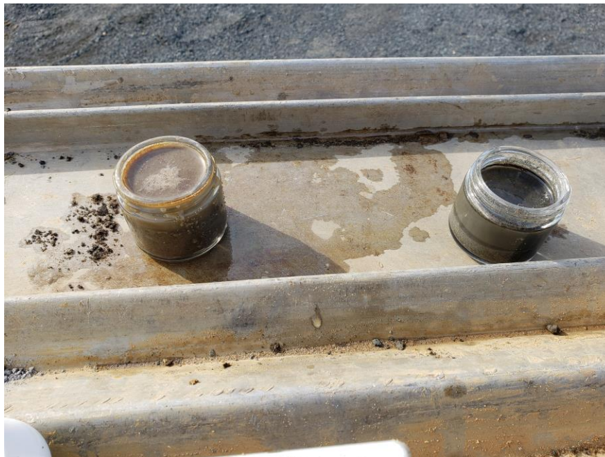
View of Failed Soil/Water Agitation Test at FPA-7 at 6.5 feet (shown right) and 8.0 feet (shown left).
