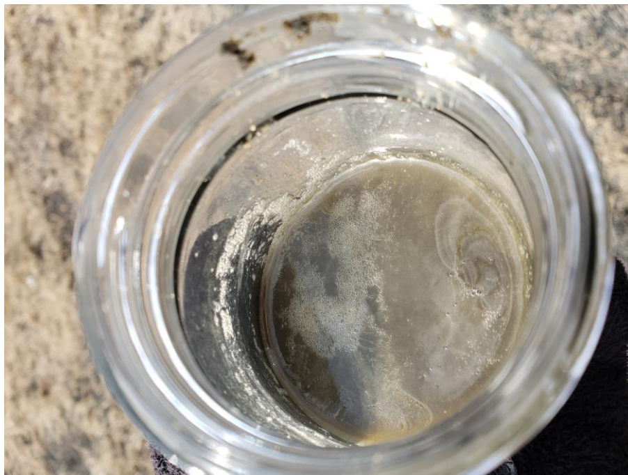
View of Failed Soil/Water Agitation Test in Boring FPA-29 at 8.0 – 8.5 Feet.
