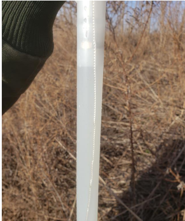
View of no measurable product on the groundwater within TWP-37.
