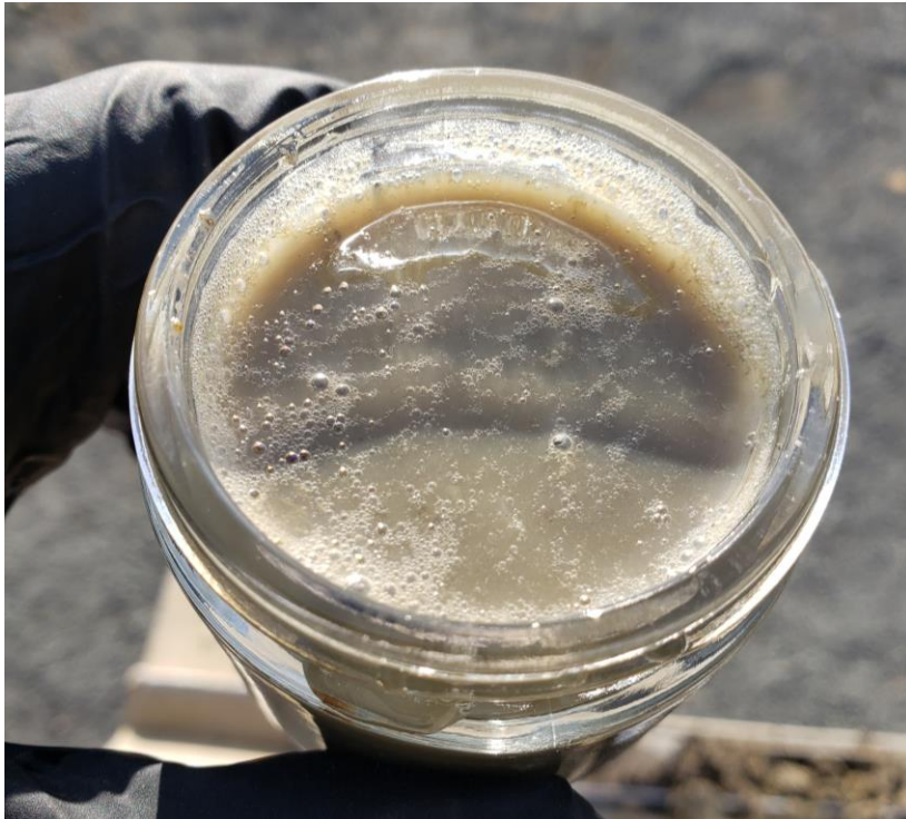
View of Failed Soil/Water Agitation Test at FPA-16 (7.0 Feet). This boring also had significant impacts in the shallow core from 1 to 3 feet below ground surface.
