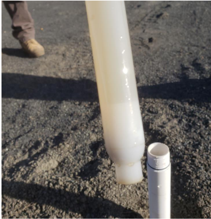
View of slight oil sheen/slick on outside of bailer at TWP-32.
