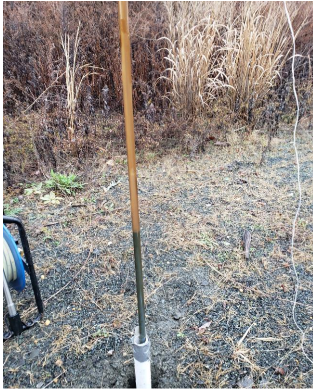
View of several feet of product in TWP-17 (Boring FPA-17). Total thickness could not be measured due to product viscosity and the bailer quality.
