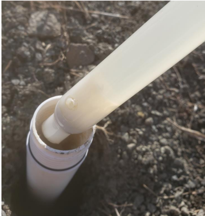
View of oil sheen/slick on outside of bailer after gauging TWP-38.
