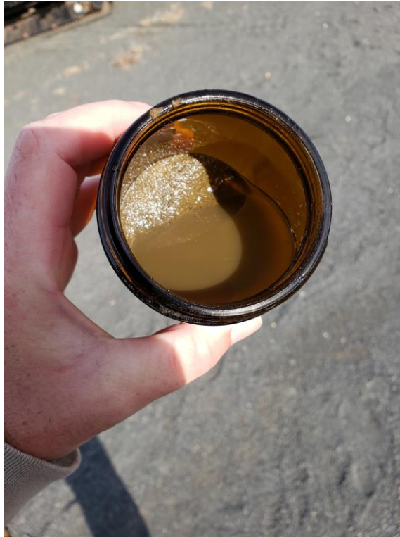
View of Passing Soil/Water Agitation Test at FPA-6. Potential Delineation Point to the south.
