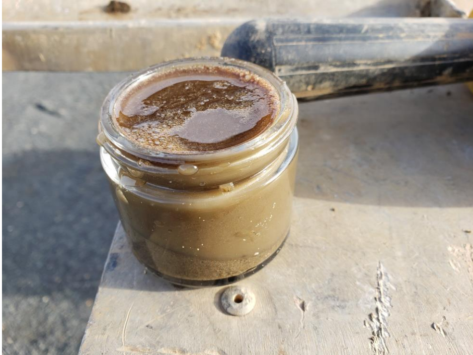
View of Failed Soil/Water Agitation Test at FPA-1 at 8.5 feet below ground surface.
