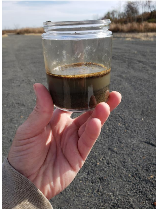
View of Failed Soil/Water Agitation Test at FPA-5 (8.5 Feet).
