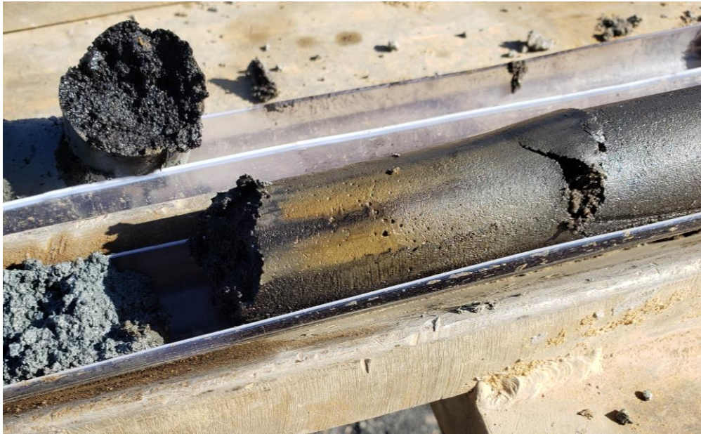
View of heavily impacted soils at 7.5 Feet within Boring FPA-22. Visible Product on soil core.
