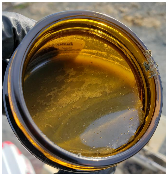
View of Failed Soil/Water Agitation Test in FPA-16 (3.0 Feet)
