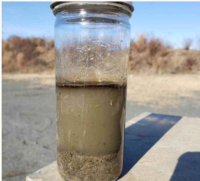
View of Failed Soil/Water Agitation Test at FPA-17 (8 Feet).
