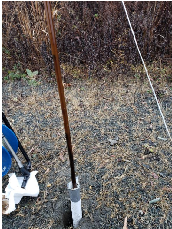
View of approximately six-inches of product in TWP-9 (Boring FPA-9).
