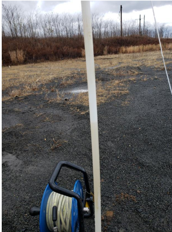
View of no measurable product at TWP-12 (Boring FPA-12). Slight sheen on groundwater and product globules/smearing on bailer.
