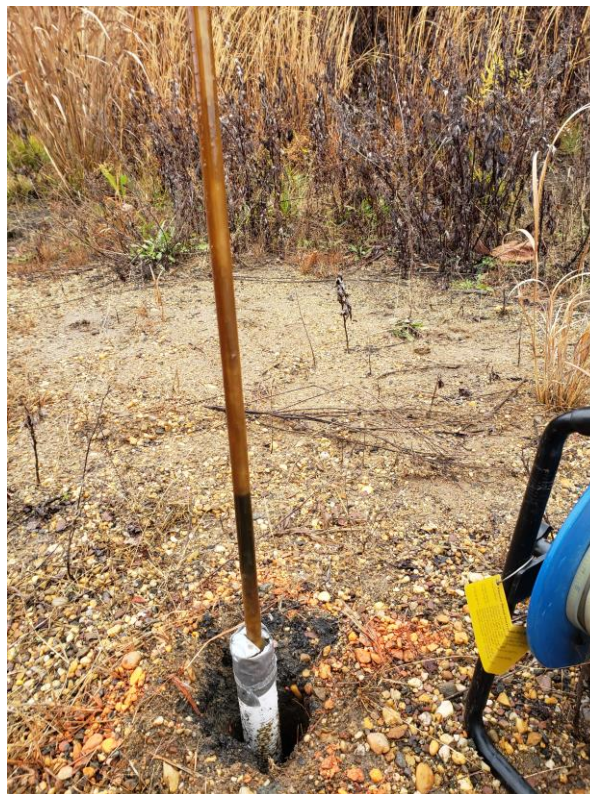
View of approximately six-inches of product in TWP-7 (Boring FPA-7).
