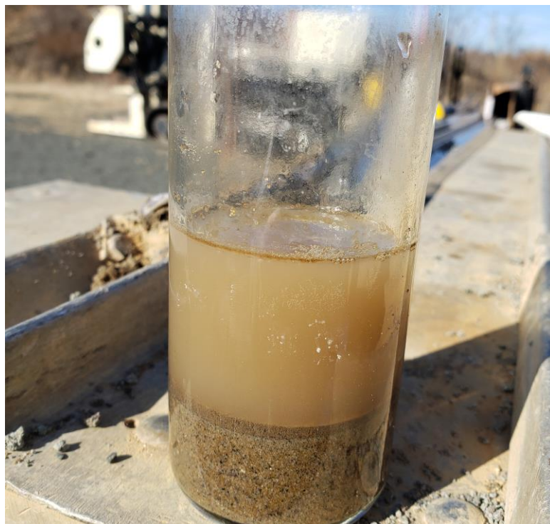
View of Failed Soil/Water Agitation Test at FPA-23 (8 Feet).
